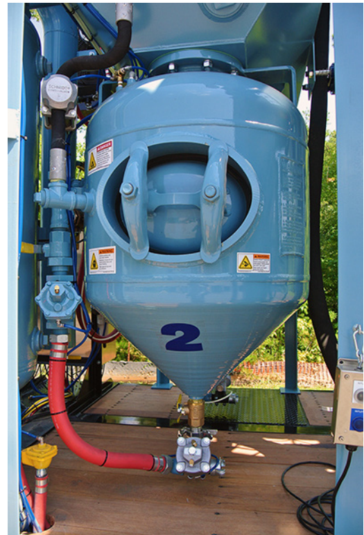
Individual pots with one outlet are much easier to use than bulk or two outlet pots.
