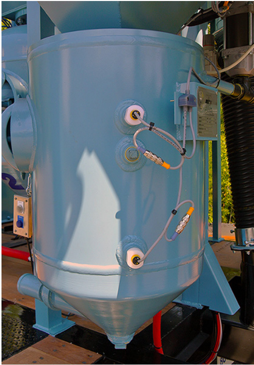
Air transfer vessels have fewer moving parts to worry about than bucket elevators and are more weatherproof.
