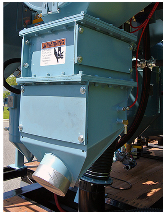
Double Dump valves provide extra discharge compartments which allows for true continuous vacuuming.
