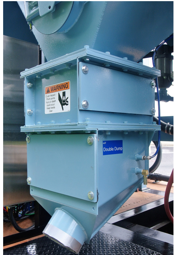
A double-dump valve is a low-cost, bolt-on assembly that can convert single-dump timer systems on vacuums and blast pots to dramatically increase production with minimal installation costs. ALL PHOTOS: © ATLANTIC DESIGN, INC.
