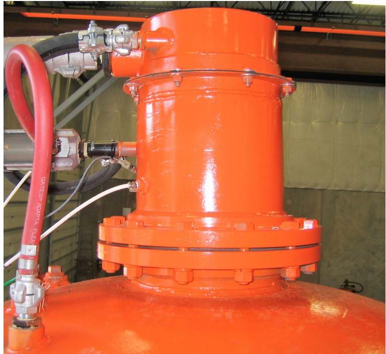
One unique high-pressure, double-dump valve application is the installation of one atop a bulk, single-chambered pot to convert it into a continuous blaster.
