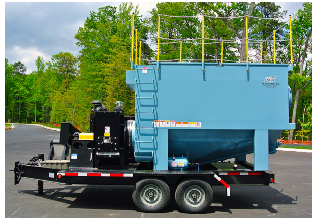
Handrails are an easy option to increase safety on a mobile dust collector.
