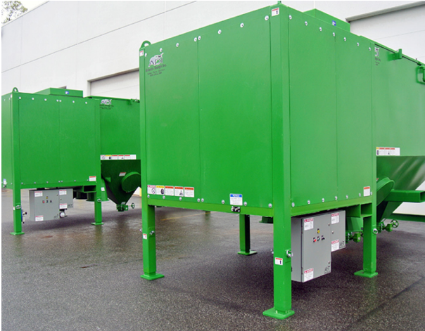
Skid-mounted units are ideal when there is no road access at a job site.
