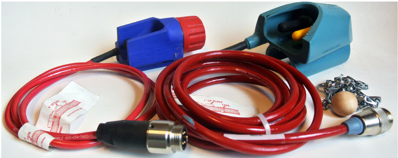
Three-wire and four-wire deadman switches provide remote abrasive cut-off/blowdown, or blast air cut-off/choke control options, that can be controlled at the nozzle instead of the blast pot.
