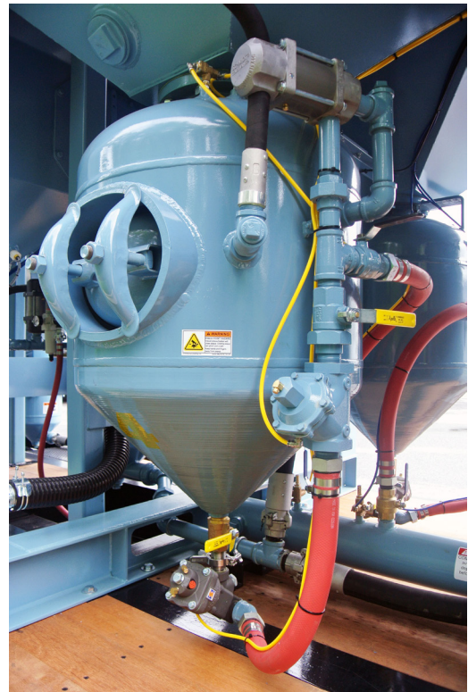
Enhanced control features allow the operator to control grit and air flow from a safer distance instead of needing to get underneath the blast pot to access the valves.
