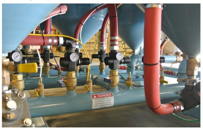
Precision blasting is enabled using blast hopper regulators to control the pressure on each individual pot.
