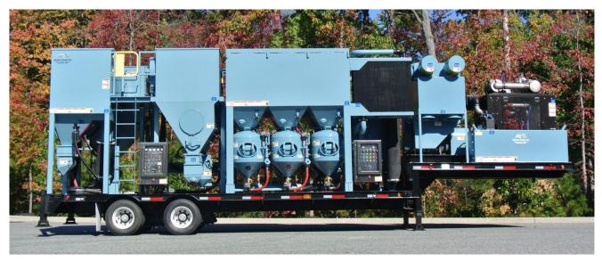
A precision-engineered blasting and reclaim machine reduces anchor patterns by controlling blasting pressure. ALL PHOTOS © ATLANTIC DESIGN, INC.
