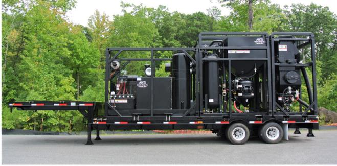
Our top of the line trailer-mounted grit blast, vacuum, and recycle systems are available in a range of models to meet your blasting needs. Combined with innovative ADI engineering, like our patented screenveyors for grit and trash separation, these machines dependably keep the worker safe and the environment clean everywhere from shipyards to bridge maintenance sites.
