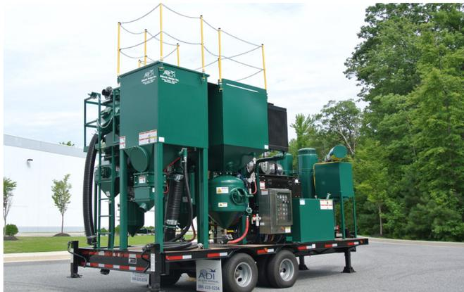
Grit Recycling Systems are used to prepare industrial surfaces for painting by grit or abrasive blasting methods.
