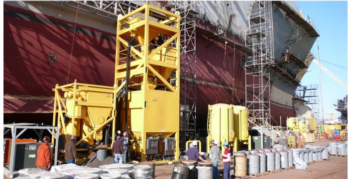
Grit Recycling Systems are used to prepare industrial surfaces for painting by grit or other abrasive blasting methods
