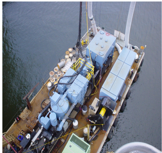
Proper ventilation and dust control is crucial for protecting the blasting personnel and the area surrounding the blast containment from excessive dust exposure. ALL PHOTOS: COURTESY OF ATLANTIC DESIGN, INC.
