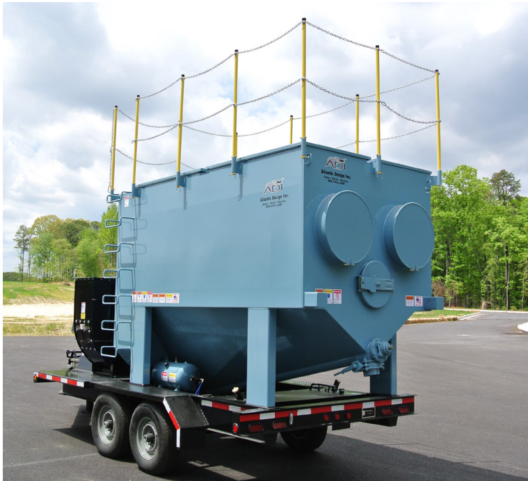
All the power required for containment ventilation systems is generated from the dust collector fan.
