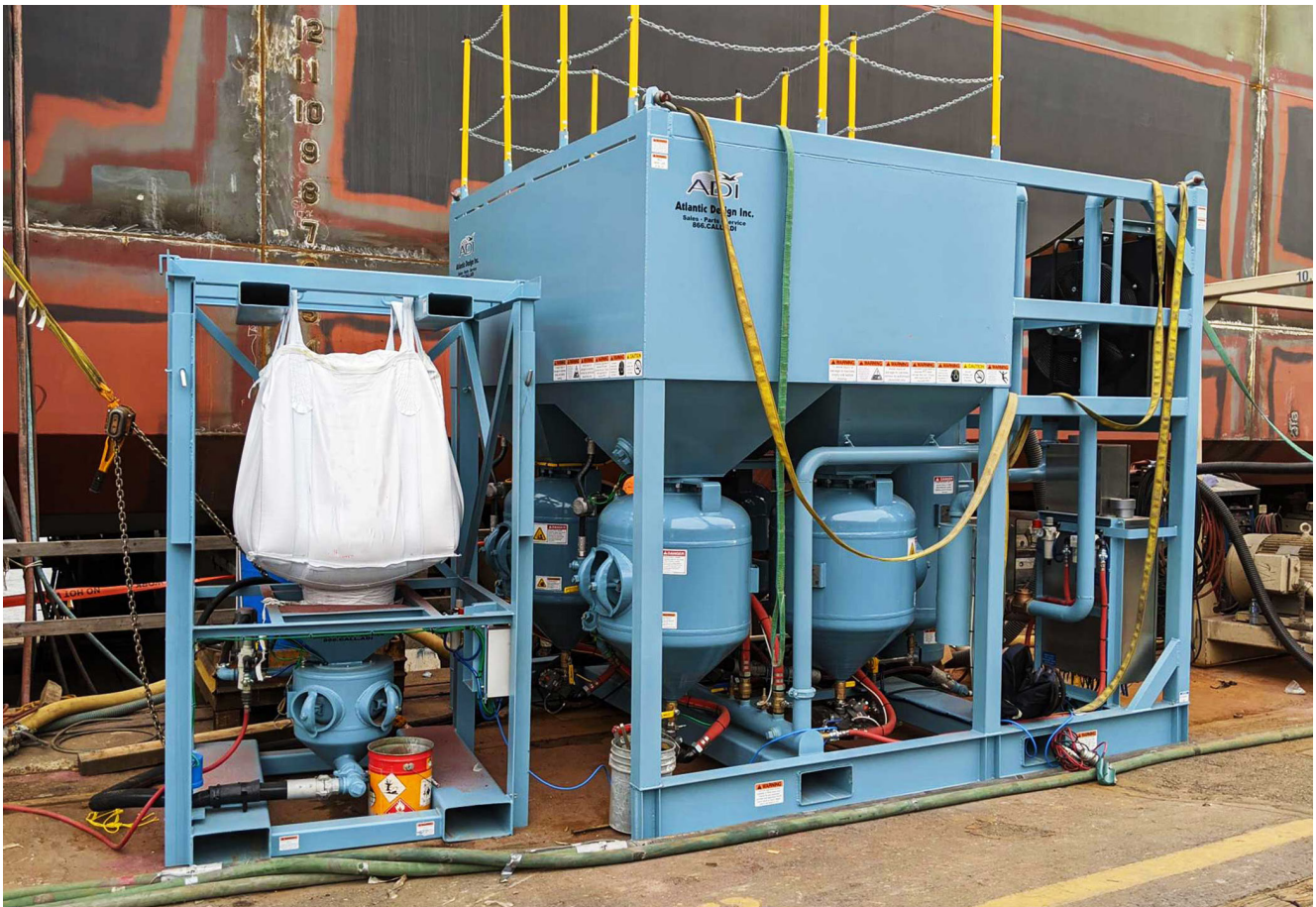
This specialty supersack loader skid can be inserted into a multi-skid system for an additional grit feed process.
