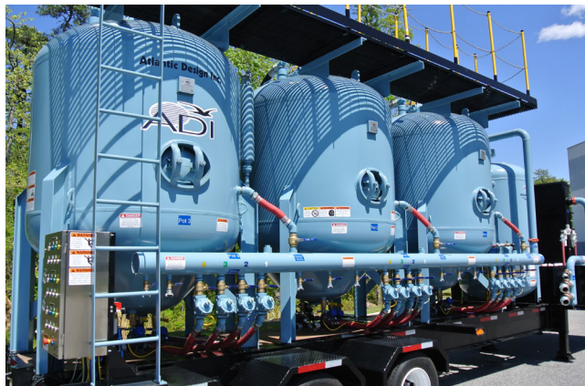
This three-pot bulk trailer, equipped with 12 nozzles, was custom-designed for remote recycling capabilities.
