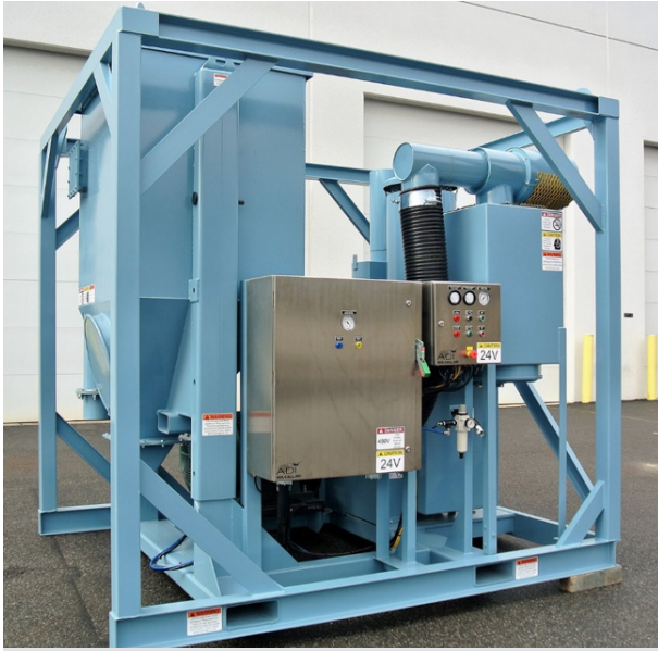
Double dump valves can increase vacuum capacity up to 25 percent.
