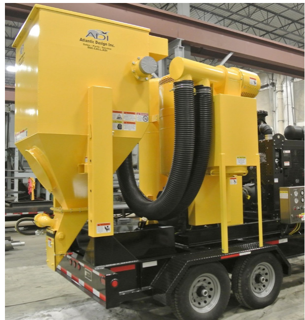
Hose and piping size should increase as they get closer to the blower.
