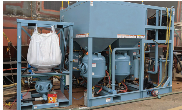
Clockwise from top left: ADI T1.5S Transfer Skid System for waste neutralizing or fresh grit additive processes; ADI Double Dump for adding a neutralizing chemical at intervals; ADI Supersack Loader with the ADI BRD430PSS unit on jobsite, using continual fresh grit media additive processing
